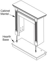
Figure 11 - Installing Cabinet Mantel onto Hearth Base
